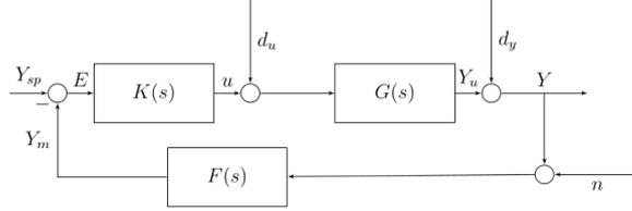
Figure 1. Block diagram of closed loop system.  $K(s)$  is the controller,  $G(s)$  is the process and  $F(s)$  is the filter.
