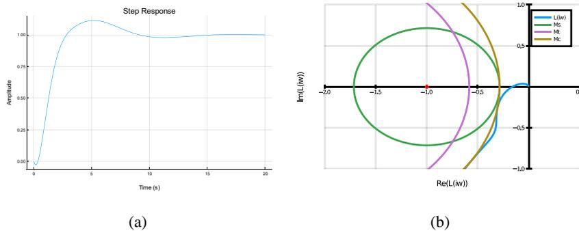
Figure 3: Step response and Nyquist plot for third order process with inverse response. HIE is used as the objective with no constraint on input usage.
