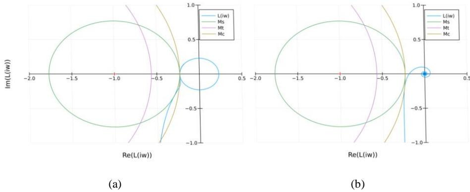
Figure 2: Nyquist plots of first order process with time delay. Left plot has constraints on maximum sensitivity and complementary sensitivity. Right plot has constraints on combined sensitivity and noise attenuation.
