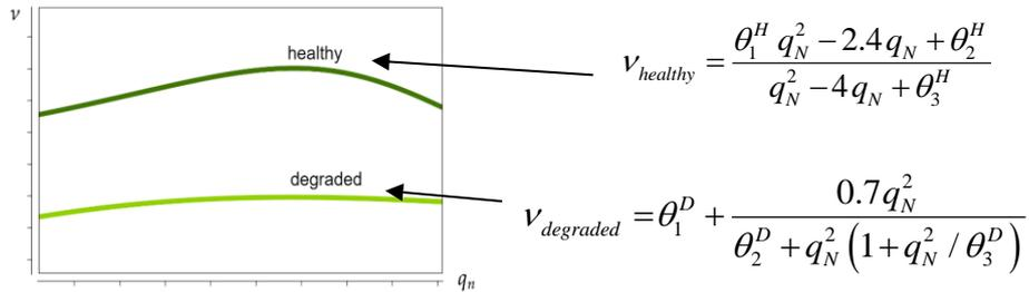
Figure 3: Compressor efficiency ( $v$ ) map as a function of compressor normalized flowrate ( $q_N$ ). To choose the estimable parameter set  $\theta^H$  and  $\theta^D$ , a sensitivity analysis was performed. The true values of the parameters are:  $\theta^H = [0.6, 2.7, 4.3]$  and  $\theta^D = [0.4, 5, 2]$ .
