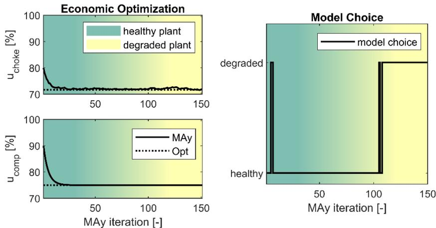
Figure 4: Tracking the true "plant" optimum (left) and the compressor degradation (right).
