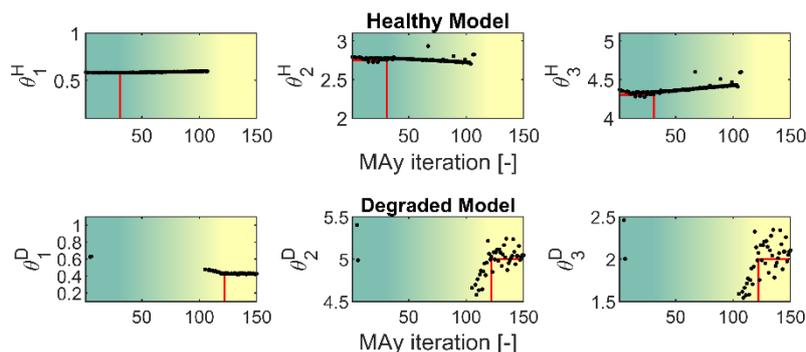
Figure 5: Estimated parameters. The red dashed line shows the true value of the parameters, while the black dots represent their estimated values (the compressor equations are shown in Figure 3).
