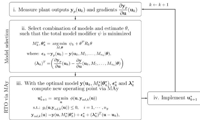
Figure 1: Simplified Diagram of the Online Model Maintenance Method
