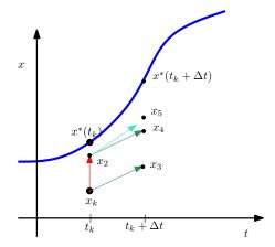
Fig. 2. Predictor, corrector, predictor-corrector, and corrected predictor steps.
