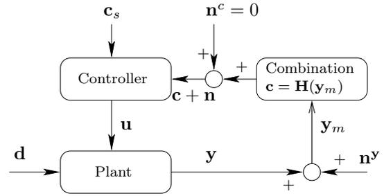
Fig. 3. Control structure (with integral action,  $\mathbf{c}_s = \mathbf{c} + \mathbf{n}$  at steady state,  $\mathbf{n}^c = 0$ )
