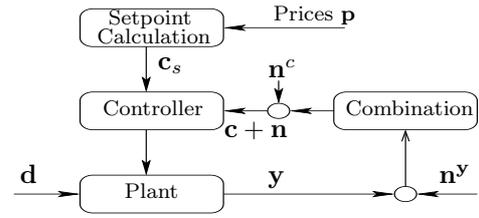
Fig. 5. Feedback control structure with setpoint calculation
