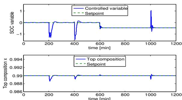
Fig. 9. Controlled variables: Self-optimizing controlled variable and top composition
