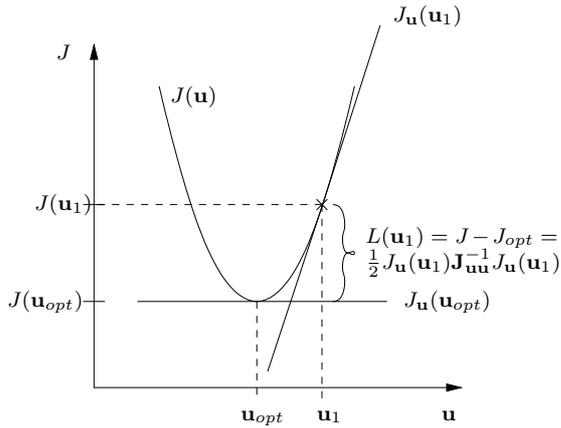
Fig. 4. Loss  $L$  imposed by non-optimal operation
