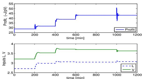
Fig. 8. Profit and inputs for the distillation column
